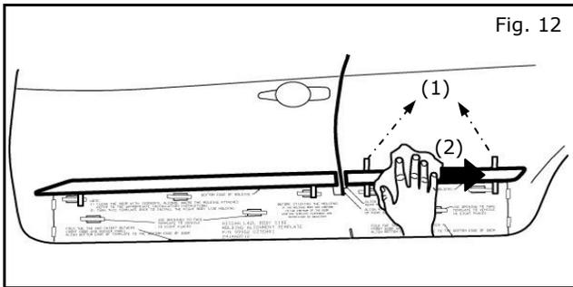
15) Align bottom edge of Rear Body Side Molding to top edge of template and press lightly into position. Slowly remove top tape liner from Body Side Molding. (See Fig. 12, Step 1)
