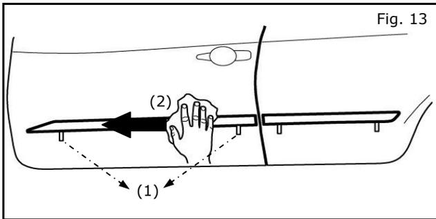
17) Remove template. Slowly remove bottom tape from Front Body Side Molding. (See Fig.13, Step 1)
