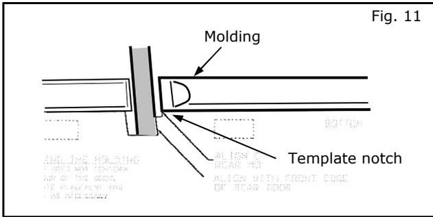
14) Align front edge of Rear Body Side Molding to template notch as shown in Fig. 11.
