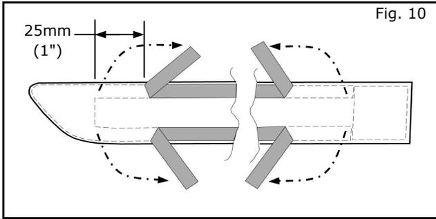
13) Peel back tape liner 25 mm (1") from all 4 ends, as shown in Fig. 10.
