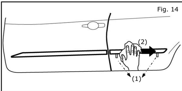
19) Slowly remove bottom tape from Rear Body Side Molding. (See Fig. 14, Step 1)
